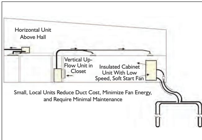
Figure 1: Options for heat pump location for simple GSHP.
