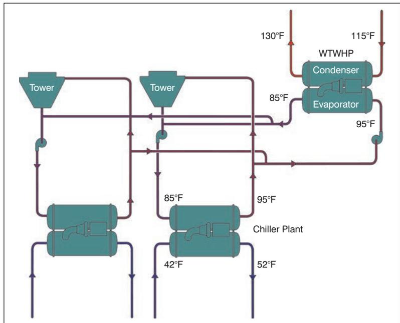
**Figure 4:** Tower water as a heat source.
