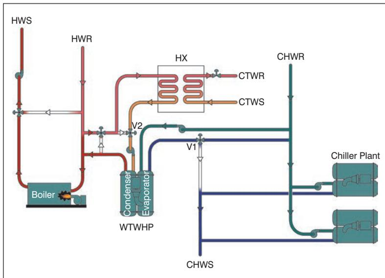
**Figure 7:** Hybrid side-stream/parallel system, operating in side-stream arrangement.
