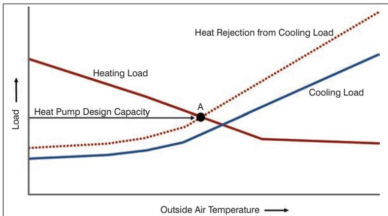
**Figure 1:** Selection point for simultaneous heating-and-cooling heat pump.
