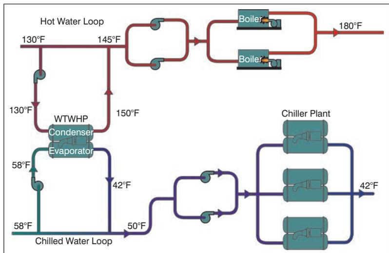
**Figure 6:** Side-stream arrangement.
