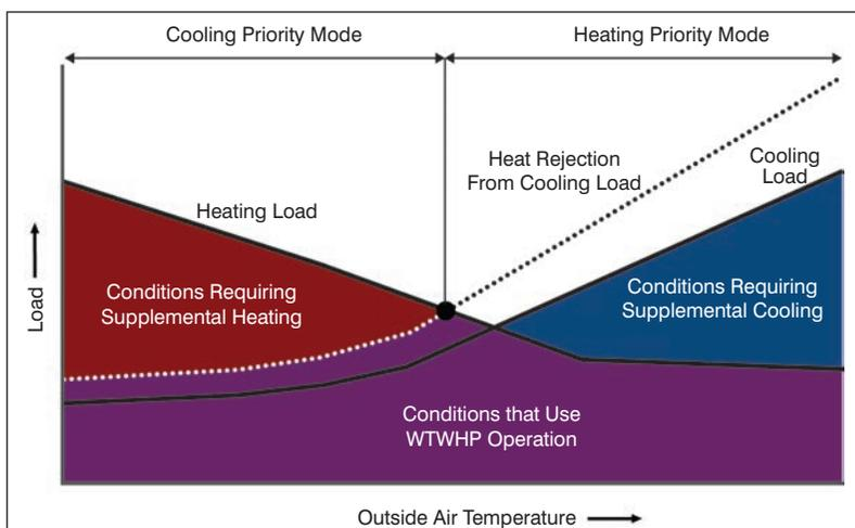
**Figure 2:** Operating areas for simultaneous heating-and-cooling heat pump.
