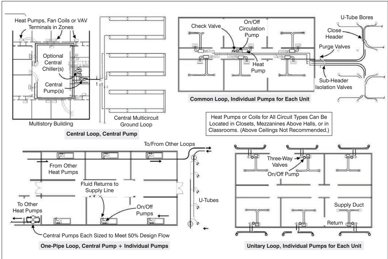
**Figure 3:** GSHP building and ground loop circuit types.
