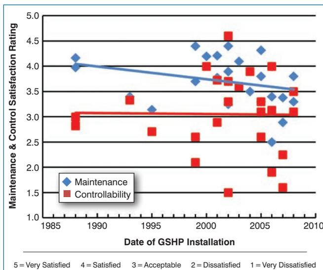
**Figure 7:** Maintenance response and controllability satisfaction vs. ground source heat pump installation date.
