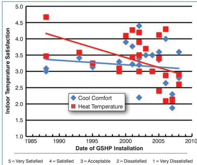
**Figure 5:** Occupant room comfort satisfaction vs. ground source heat pump installation date.
