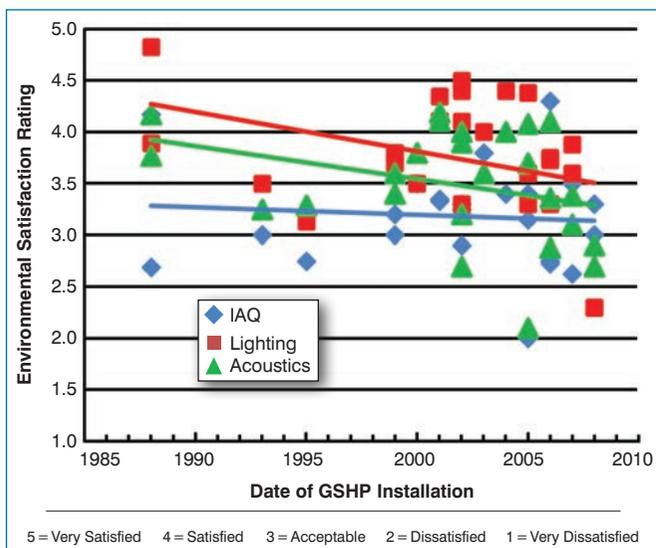
**Figure 6:** Occupant IAQ, lighting and acoustic satisfaction vs. ground source heat pump installation date.
